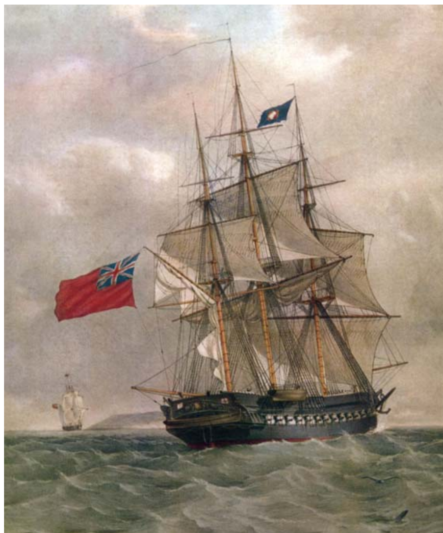
HMS Pomone , launched in 1805, was a 38-gun 18-pdr Leda-class frigate. More Leda-class frigates were built for the Royal Navy than any other frigate design. (AC)
