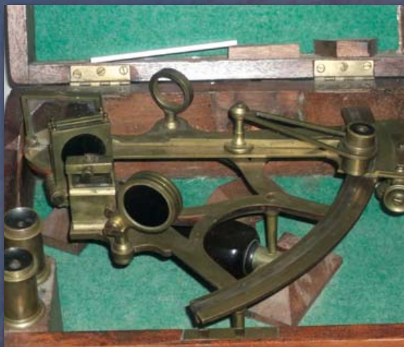
A naval sextant, used to determine local noon during the age of fighting sail. [AP-HMM]
